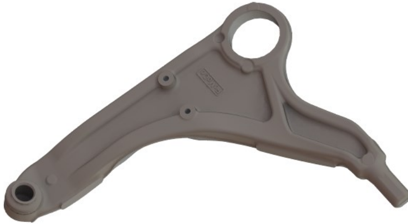
Figure 1: Ford Baseline LH Control Arm Design
