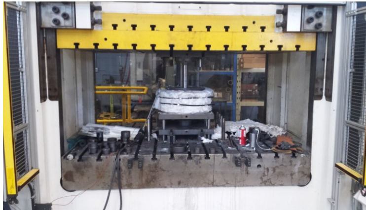
Figure 5: 1200-Tonne hydraulic press at CanmetMATERIALS [17]
