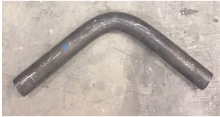
Figure 18: Preform: 63.5mm dia. x 716mm extruded AZ80 bar stock with a 108° bend angle
