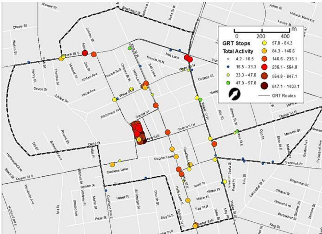
Figure 4-4. Bus stop activity in Downtown Kitchener
