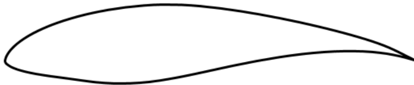
Figure 2.6 S826 airfoil shape.
