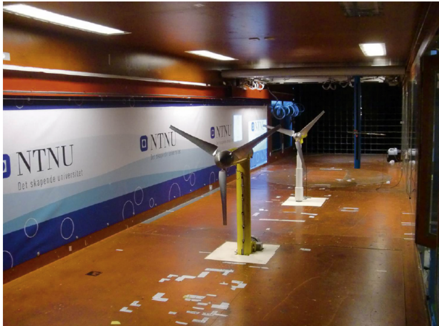
Figure 2.16 The tandem-wind-turbine experiment [1].
