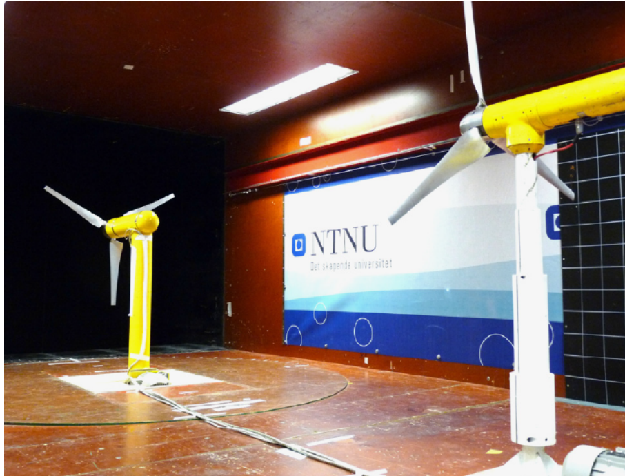
Figure 2.23 The two staggered wind turbines in Krogstad wind tunnel experiment [2].
