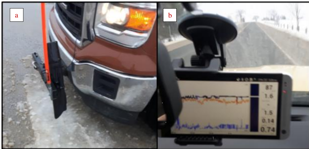
Figure 3.4: Teconer system installed on the MDCU
