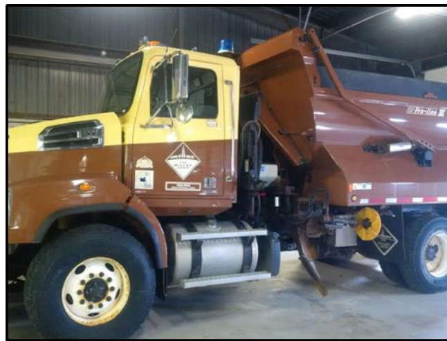
Figure 3.3: Vehicle used for spreading winter road maintenance materials
