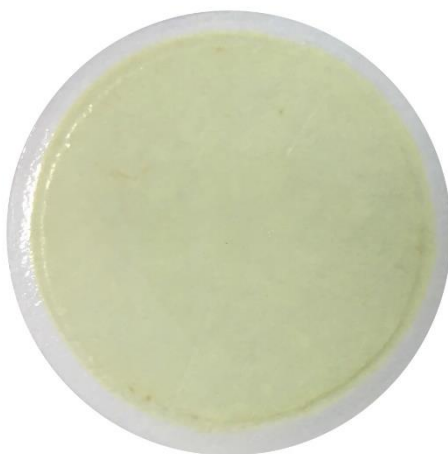
Figure 4.10 Photograph of the used NF membrane after cleaning by water washing.
