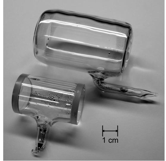
FIG. 4. Two  $^3\text{He}$  cells. The larger of the two cells, called Skylight, was used in the polarimetry measurements. The smaller flat-window cell called Pistachio was used as a target cell. Rubidium deposits can be seen as dark spots along the walls of the cell.
