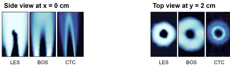
Figure 6.17: Comparison of the Bunsen flame profiles from LES, BOS tomography for f/16 images, and chemiluminescence tomography. Side and top view cross sections are presented for x = 0 cm and y = 2 cm, respectively, showing close correspondence of the flames.
