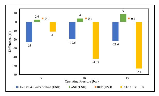
Figure 5.4 Breakdown of Difference between Atmospheric and Pressurized Power Plants in the US in terms of Bare Module Costs
