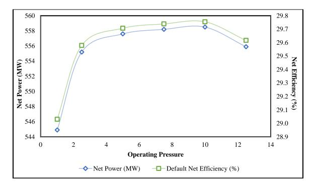
Figure 4.2 Net Power and Efficiency as a Function of Operating Pressure
