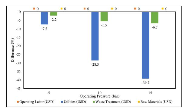
**Figure 5.5** Breakdown of Difference between Atmospheric and Pressurized Power Plants in the US in terms of C<sub>OL</sub>, C<sub>u</sub>, C<sub>WT</sub> and C<sub>RM</sub>
