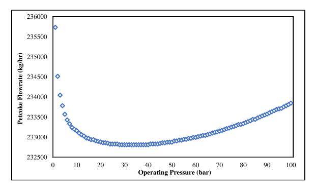
Figure 4.3 Petcoke Flowrate as a Function of Operating Pressure
