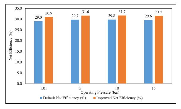
Figure 4.10 Default and Improved Net Efficiencies at Various Operating Pressures
