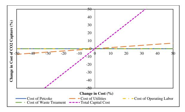
Figure 5.15 Sensitivity Analysis of the Cost of CO<sub>2</sub> Capture in KSA
