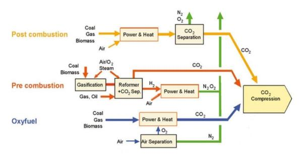
Figure 1.2 Overview of Carbon Capture Processes (IPCC, 2005)
