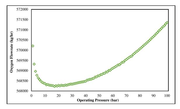
Figure 4.4 Oxygen Flowrate as a Function of Operating Pressure
