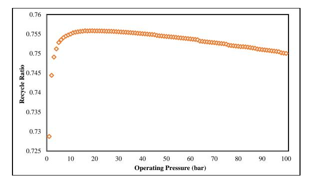
Figure 4.5 Recycle Ratio as a Function of Operating Pressure
