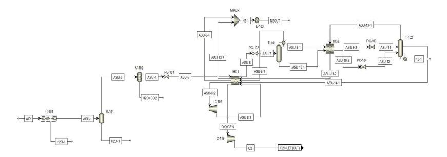
Figure 3.3 Air Separation Unit Flowsheet
