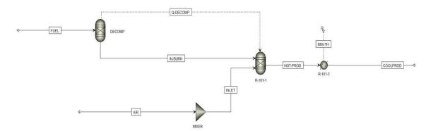
Figure 3.2 Conventional Air-Fired Combustion System for Coal and Petcoke
