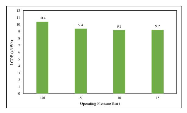
Figure 5.1 LCOE for Oxy-Petcoke Power Plant in the US at Various Pressures
