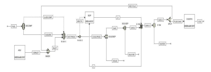
Figure 4.8 Modified Oxy-Combustion Process Flowsheet
