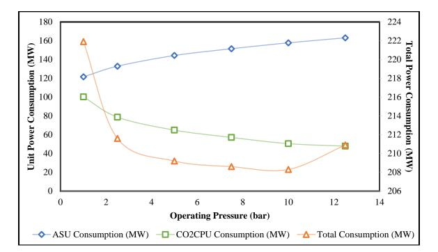
Figure 4.1 Power Consumption as a Function of Operating Pressure
