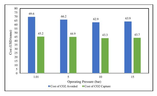
**Figure 5.2** Cost of CO<sub>2</sub> Avoided and CO<sub>2</sub> Capture for Oxy-Petcoke Power Plant in the US at Various Pressures
