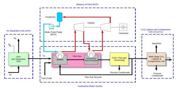
Figure 1.3 Typical Oxy-Fuel Power Plant (Shafeen, 2014)
