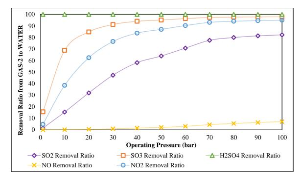
Figure 4.6 Impact of Pressure on SO<sub>x</sub> and NO<sub>x</sub> Removal
