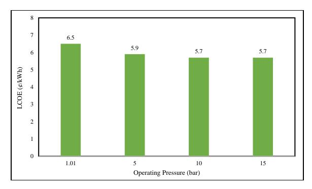
Figure 5.6 LCOE for Oxy-Petcoke Power Plant in KSA at Various Pressures
