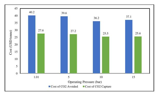
**Figure 5.7** Cost of CO<sub>2</sub> Avoided and CO<sub>2</sub> Capture for Oxy-Petcoke Power Plant in KSA at Various Pressures
