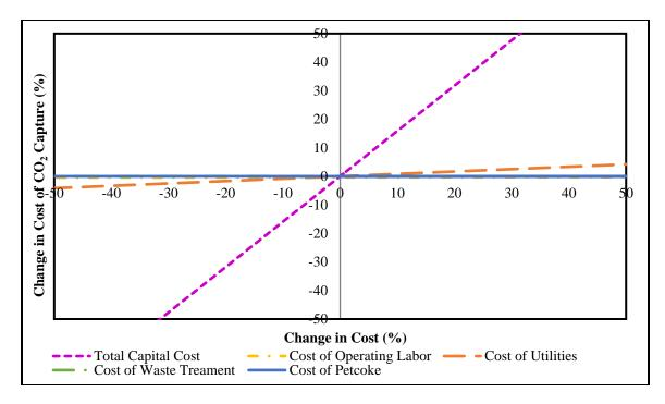
Figure 5.11 Sensitivity Analysis of the Cost of CO<sub>2</sub> Capture in the US
