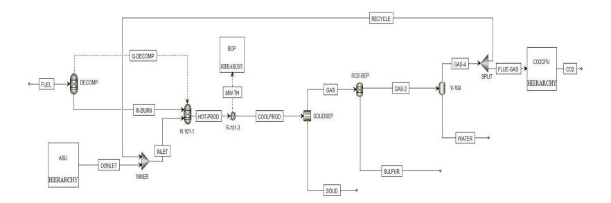
Figure 3.1 Oxy-Combustion Process Flowsheet for Coal and Petcoke
