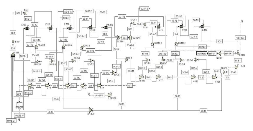
Figure 3.4 Balance of Plant (Steam Cycle) Flowsheet
