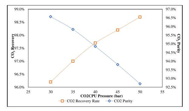
Figure 4.7 Impact of CO2CPU Operating Pressure on CO2CPU Performance
