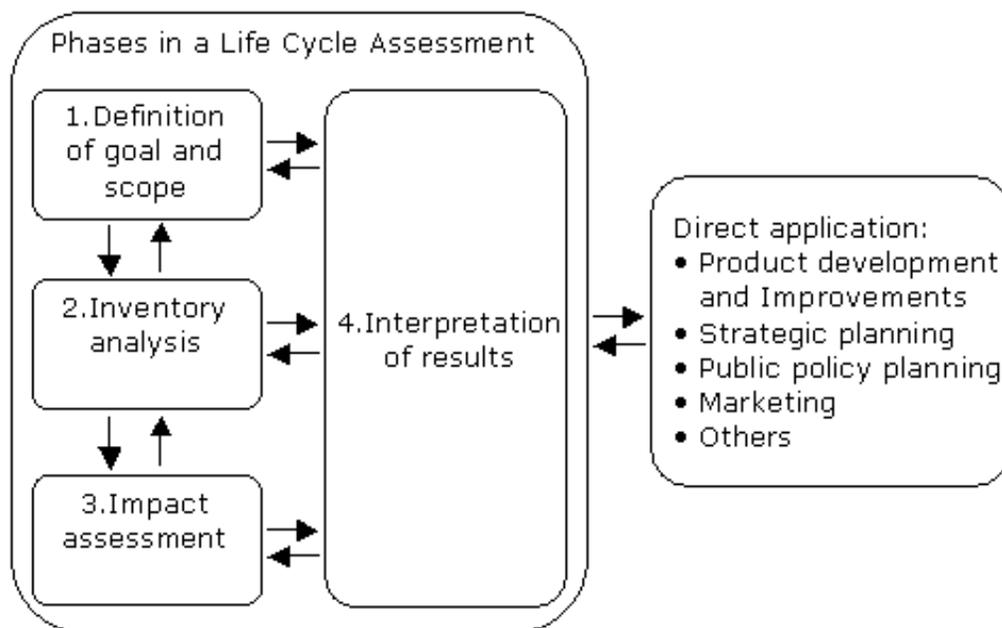
Figure 2: shows the LCA methodology steps (Bayer et al, 2010).
