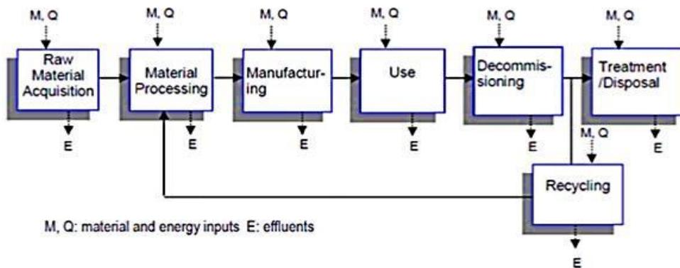
Figure 4: Life Cycle diagram of PV system (Frishknecht et al., 2012)
