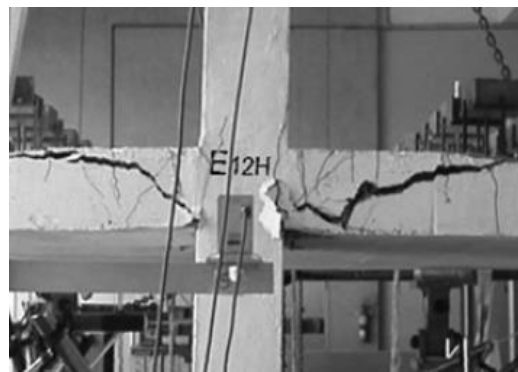
Figure 2-5: Inclined Shear Cracks in Slab After Punching Failure (Anggadajaja & Teng, 2008), authorized reprint from ACI Structural Journal, Volume 84, Issue 3, 2008
