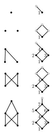
Figure 3.3: An example of decoding the lattice with covering sequence (2,0,0,2,0,0,1,0). The improved compression code is the bitstring 1000100000, in which three ones are omitted compared to the simple compression code. The numbers give the order in which the nodes are visited (as determined by **Rule**), and open circles indicate unvisited nodes.
