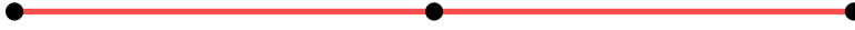
Figure 6.31: Pictorial representation of global DOFs on the unit interval [0, 1] with respect to the triangulation [0, \frac{1}{2}] \cup [\frac{1}{2}, 1] . Solid dots mark the points associated to the global DOFs.
