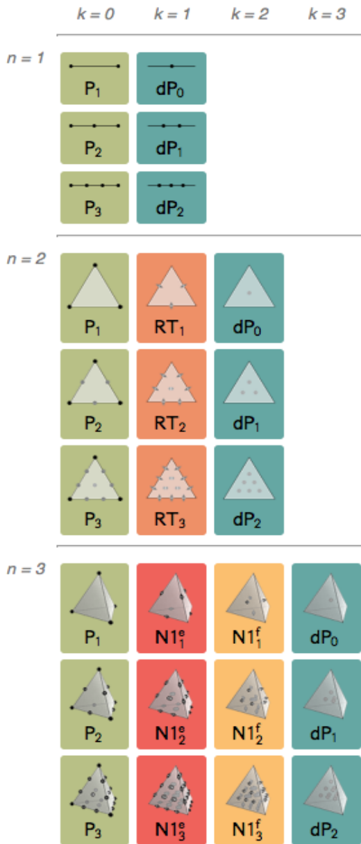
Figure 9.53: The first two columns of the Periodic Table of the Finite Elements. Cohomology-preserving families of finite element spaces are arranged horizontally in the first column and diagonally in the second column.
