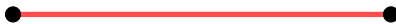
Figure 6.21: DOFs for the Lagrange finite element in Example 6.2.3. Solid dots represent the points p such that \text{eval}_p is a DOF.
