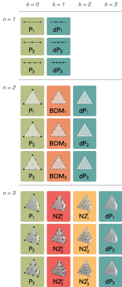
Figure 9.53: The first two columns of the Periodic Table of the Finite Elements. Cohomology-preserving families of finite element spaces are arranged horizontally in the first column and diagonally in the second column.
