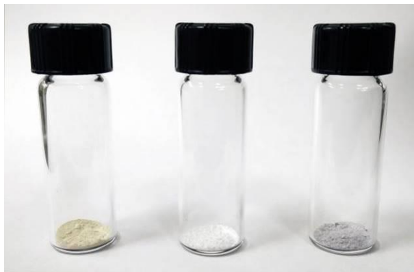
Figure 6-3. Optical image of (from left to right) Ag-TiO 2 before heat treatment, pure TiO 2 after heat treatment, and Ag-TiO 2 after heat treatment.
