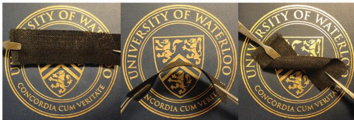
Figure 4-6. Optical images showing (from left to right) light transmission, bending, and twisting of the as-prepared electrode.
