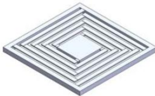
Figure 6 The quad-folded design with n=4 , where "n" is the number of turns of folded spring [27]. Courtesy of Paprotny et al., Micro Nanotechnology Power Generat. Energy Convert. Appl.
