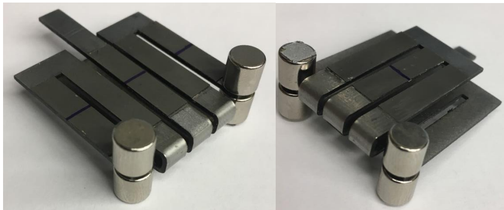
Figure 23 Manufactured unit showing the polarization of PZT strips along with the top and bottom isometric view
