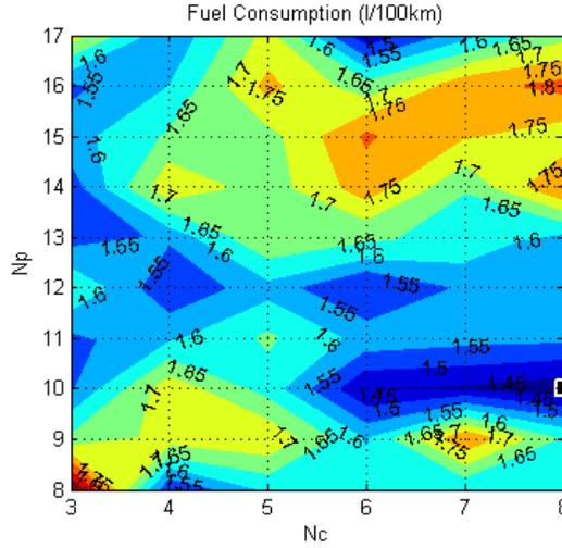
It can be seen that the least fuel consumption can be found with  $N_c = 8$  and  $N_p = 10$ . All simulations have been done with respect to these values. Therefore fuel economy will not necessarily be improved by increasing prediction horizon.
