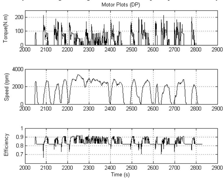
Figure 12. Dynamic Programming result: Generator Torque, Speed, Efficiency
