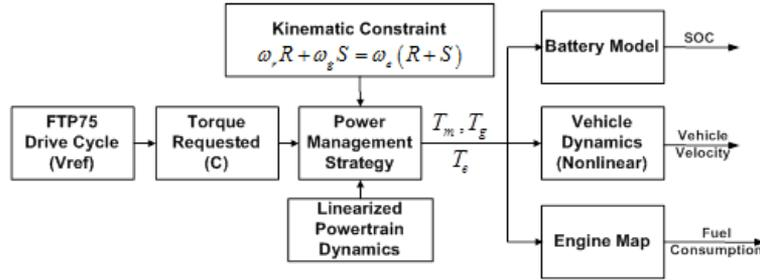
The battery is fully charged at the beginning of the drive cycle and the vehicle goes on a pure electric mode until the state of charge drops to 0.3, the reference state of charge. Fuel consumption in this period is zero.
