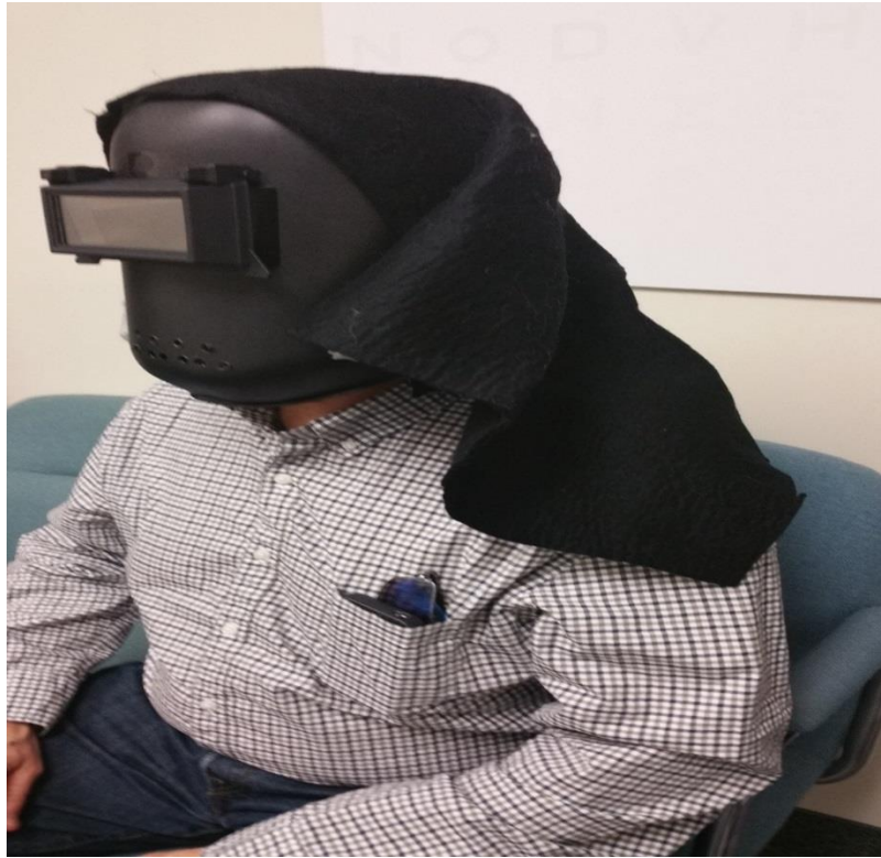
Figure 3-4: A participant wearing welding helmet with filter in front of eyes in order to reduce the light level.
