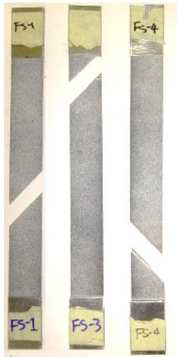
Figure 61. Failure surfaces of in-plane shear specimens.
