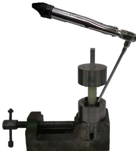
Figure 38. Combination of Allen key and torque wrench used to tighten the locking assembly.
