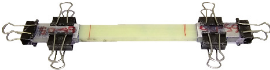
Figure 40. Binder clips used on a coupon to ensure a uniform adhesive bondline.
