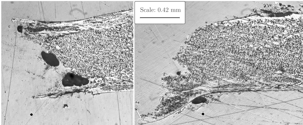
Figure 71. Static shear failure surface in tubes.
