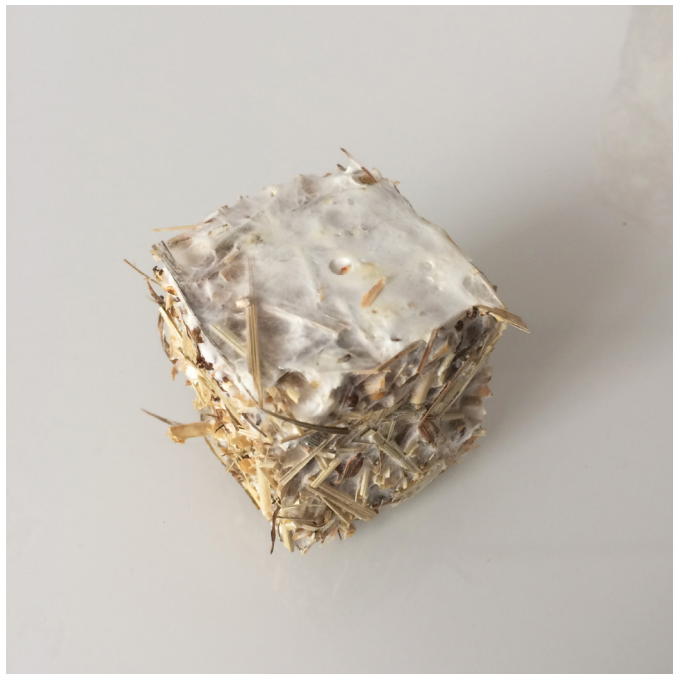
Fig. 29 Mycelium Colonizing Straw Sample removed from mould 8 days after inoculation.
