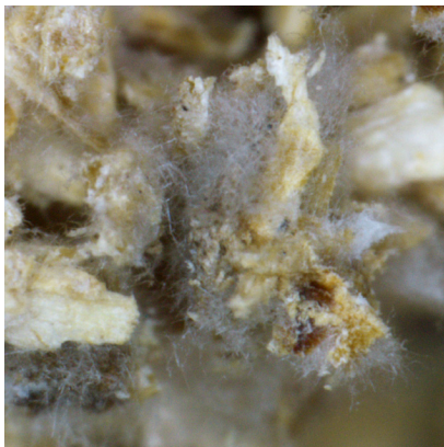
Fig. 07 Microscopic Image Zoom Sawdust fragments colonized by mycelial network- zoom.
