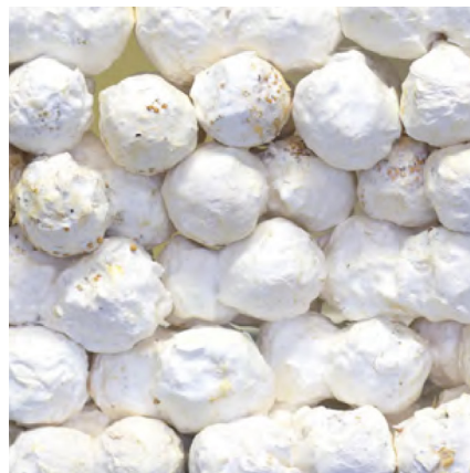
Fig. 20 Sean Campbell et al., Modular Mycelia Elements fusing to create a larger assembly
