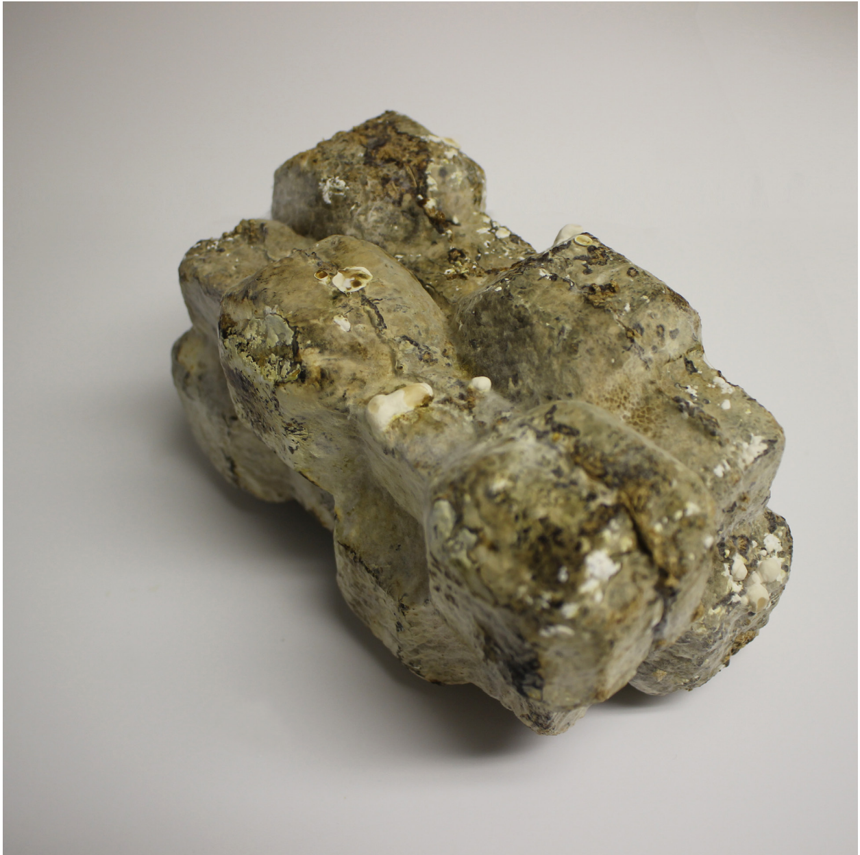
Fig.96 Hyphal Bonding as Joinery Fusing as means of assembly. Same logic as projects: Mycotecture and Modular Mycelia
