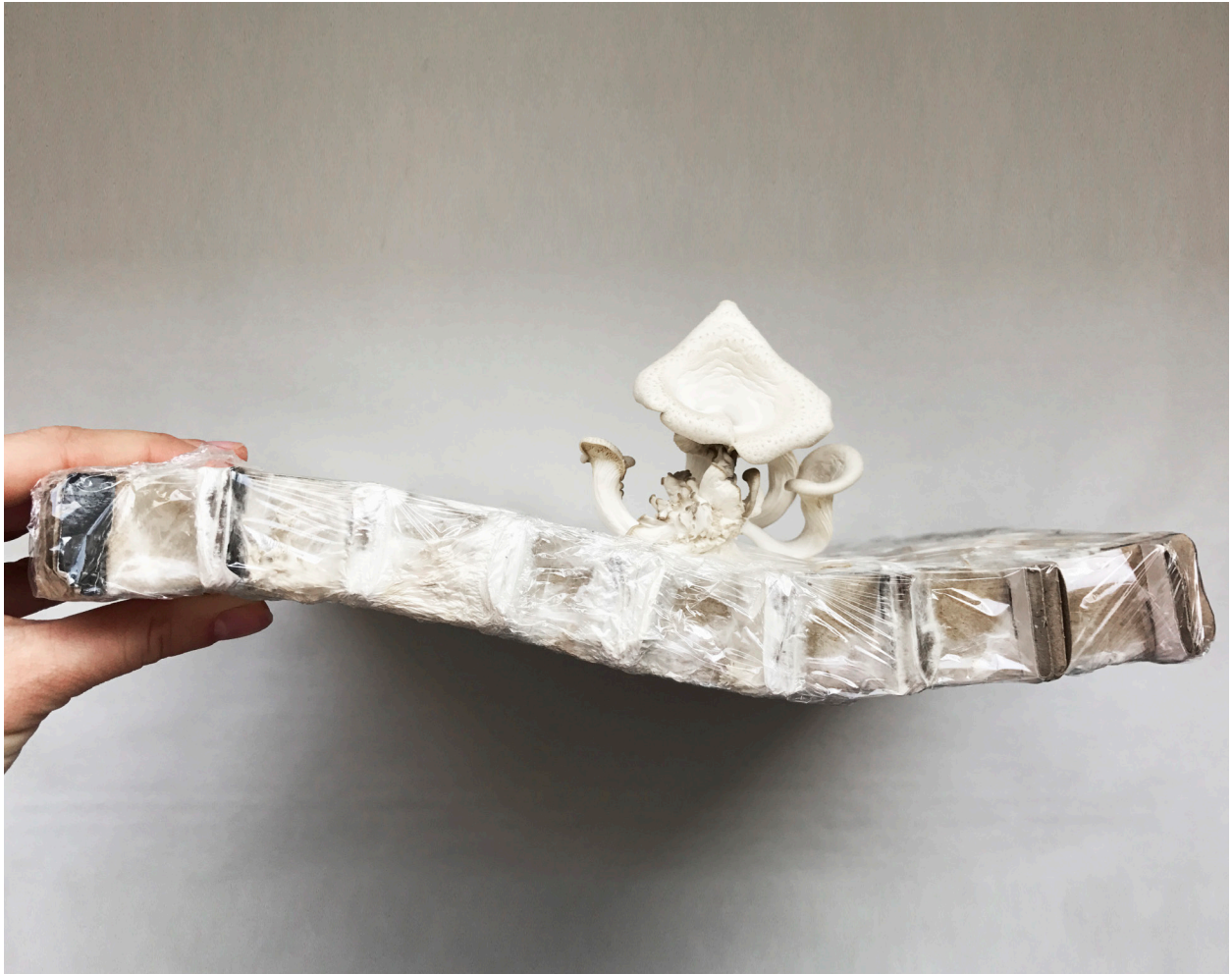
Fig. 40 Cardboard Waffle Structure Internal Scaffolding
