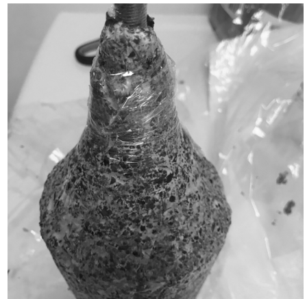
Fig.103 Testing Intricate Moulds Bandaging damage for self-repair
