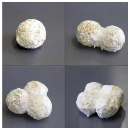
Fig. 19 Sean Campbell et al., Modular Mycelia Spherical elements fusing
