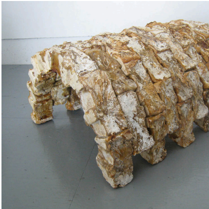
Fig. 13 Phil Ross, Mycotecture Blocks fusing to create continuous structure
