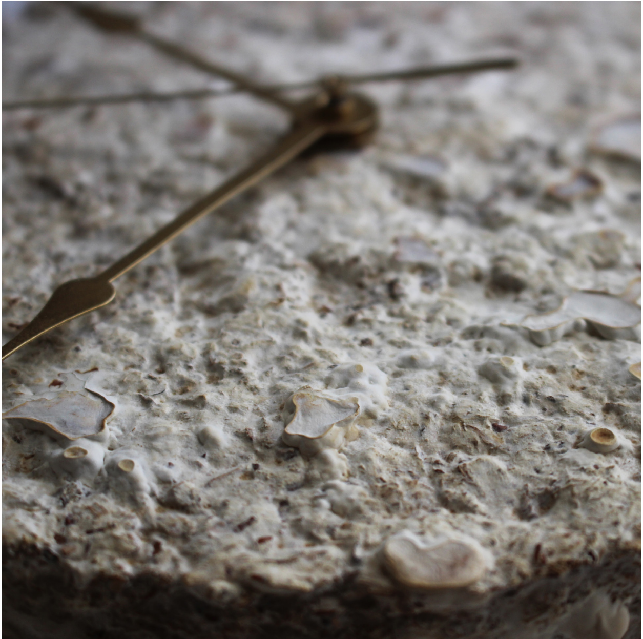
Fig.101 Material Learning Through Prototyping Artifact was able to self-heal, leaving no trace of damage
