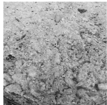
Fig.99 Cracks Object in process of curing and self-repair
