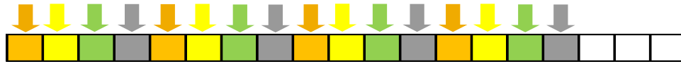
Figure 3.2: Parallel full table scan (PFTS) in SAP SQL Anywhere. Each color represents a different worker.
