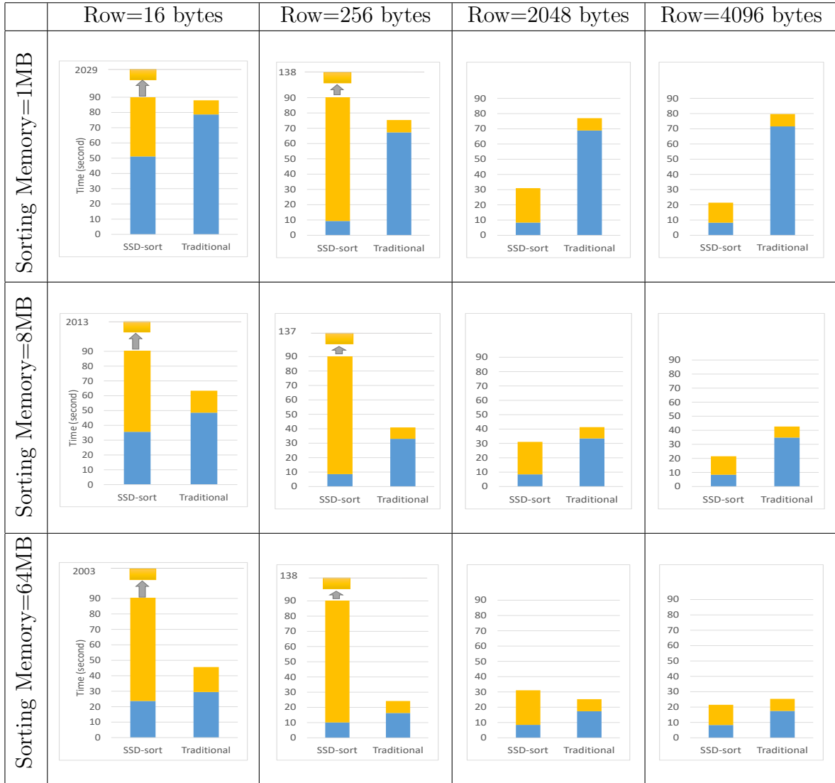
Figure 4.4: The execution time of SSD-sort vs. that of the traditional method when the memory buffer pool size is 50% of the input size. In each graph, the blue color represents the time-to-first-row, and the orange color represents the fetch time.
