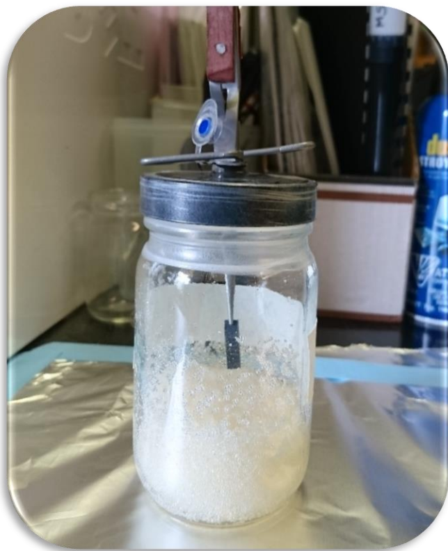
Figure 6.1: A 250 mL McReynolds standard headspace generating jar being sampled from with a TF-SPME device held by cross-locking tweezers.
