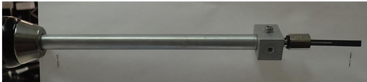
Figure 4.3 Modified power drill set-up holding a 4 cm x 5 mm DVB/PDMS/carbon mesh TFME membrane.
