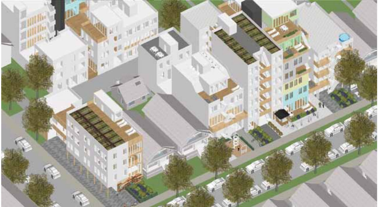
Figure 3.9.3: The shift of exterior recreational space to roof tops from backyards and high visibility of stairs.
