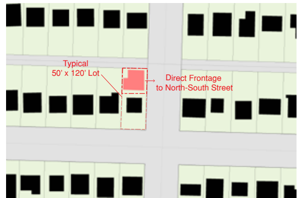
Figure 2.7.20: Plan of corner condition which allows for property subdivision along north-south street.
