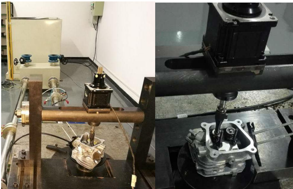
Figure 4.8 Cylinder head inlet and outlet flow tests for flow coefficient identification at different valve lifts
