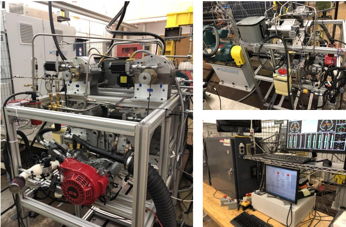
Figure 7.5 Overall set up of the HVVA engine test bench
