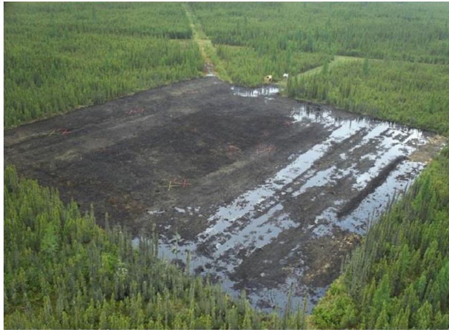
Figure 1-1 Well-pad after peat replacement treatment ( http://www.nait.ca/70709.htm ).
