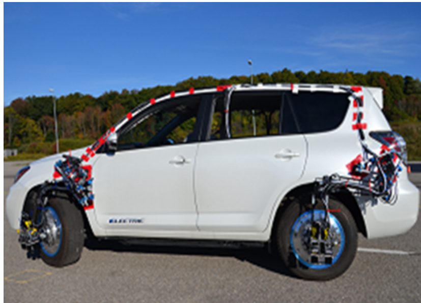
(a) Rav4EV instrumented with measurement system
