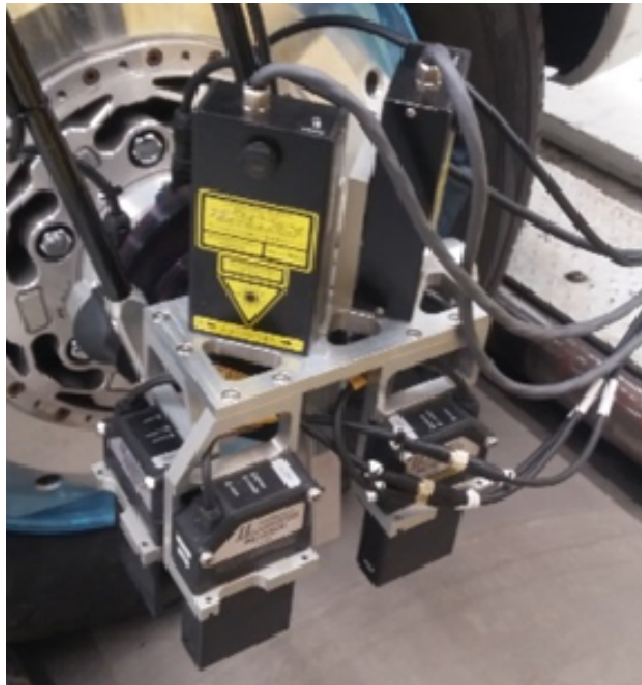
Figure 2.4: LGS and LDV sensor set mounted on wheel hub
