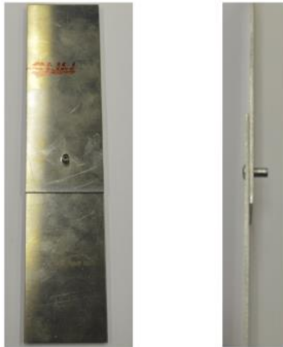
Figure 93: Lap shear specimen with 5 kN rivet
