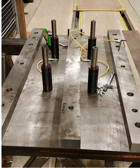
Figure 19: Nitrogen springs mounted on the die platform
