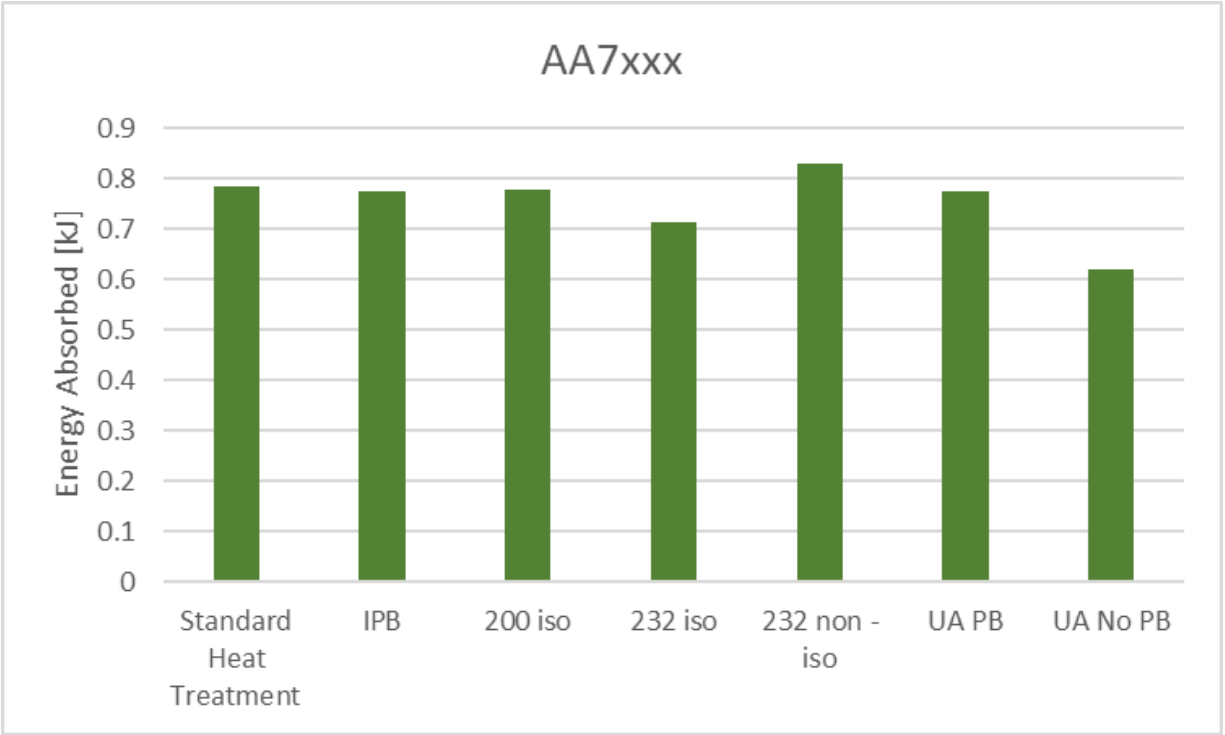
Figure 90: Energy absorbed comparison between warm forming and die quenching for AA7xxx
