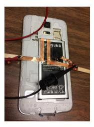
Figure 3.4: Bypassing the Battery
