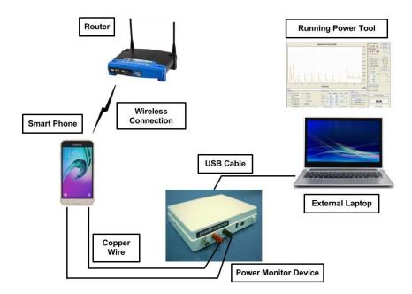
Figure 3.3: Experimental Setup for detecting Malware using Power Signatures
