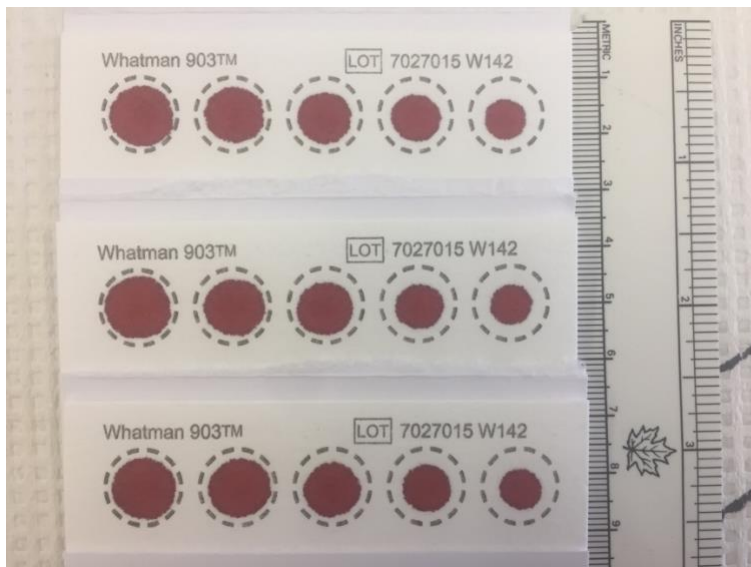
Figure 3. Whole blood spotted on 903 Protein Saver Cards. Volumes of 35, 30, 25, 20 and 15 \mu L were pipetted into the center of each spot and areas were determined using ImageJ.
