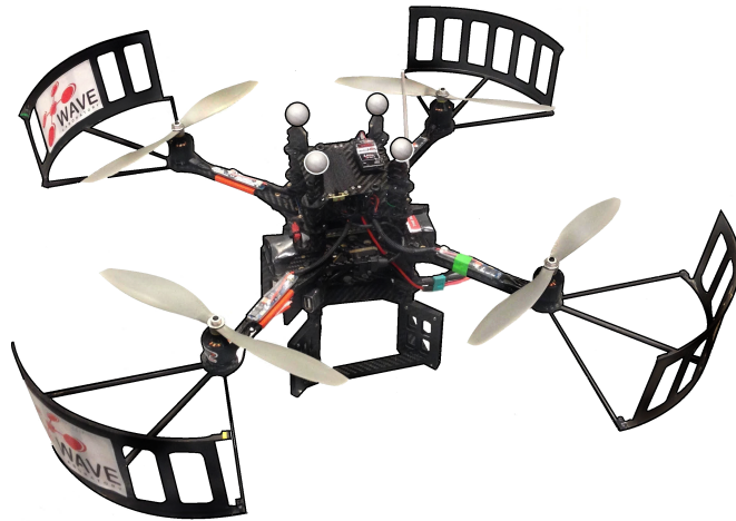
Figure 4.3: The AscTec Pelican quadrotor used for collecting the quadrotor dataset.
