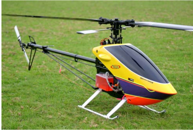
Figure 4.8: The Synergy N9 helicopter vehicle used in the Stanford helicopter dataset.
