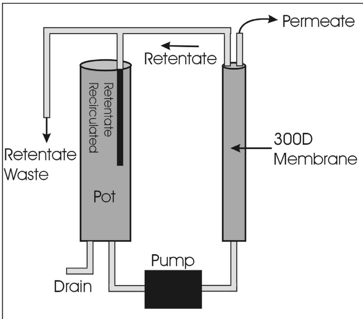
Figure 4. Detailed schematic diagram of reverse osmosis apparatus.
