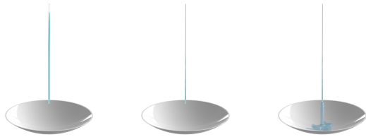
Fig. 12. Reduced-liquid flow and dripping on a single strand. Left: No reduced-liquid flow. Center: Reduced-liquid flow without dripping; the liquid flows towards the tip and disappears. Right: Reduced-liquid with dripping enabled.
