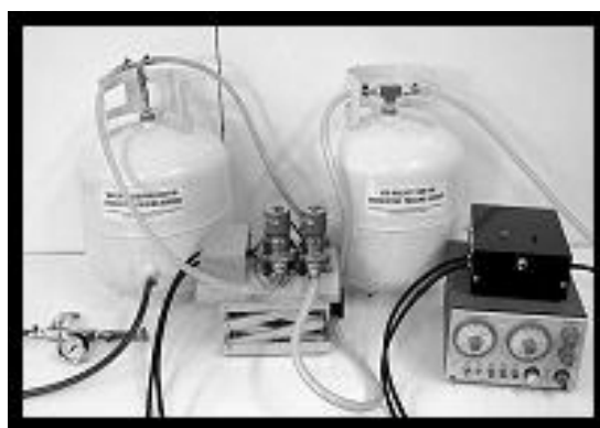
Figure A.4: The compressed-gas CPS. The two tanks are the water reservoir and air accumulator. The two solenoid valves control air pressure in the water reservoir. Finally, there is a square-wave generator with a relay box on top of it, this controls the solenoid valves.
