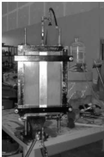
(c) Filled experimental cell with compression bracket
