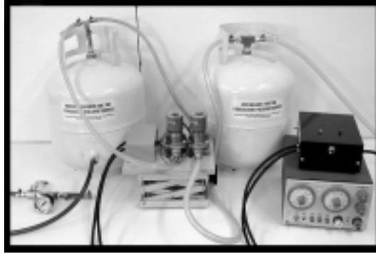
Figure 3.4: The compressed-gas CPS. The two tanks are the water reservoir and air accumulator and the two solenoid valves are for controlling air pressure in the water reservoir. Finally, there is a square-wave generator with a relay box on top of it that controls the solenoid valves. The square-wave generator was eventually replaced by a computer.
