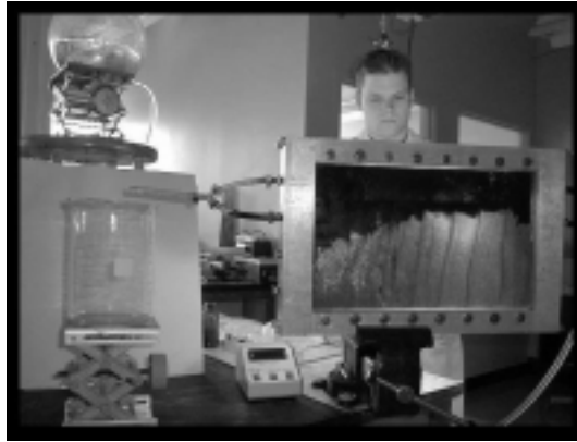
Figure E.1: Lab setup. The air has a slightly silver colour in this picture. Note the location of the inflow/outflow ports into the cell.
