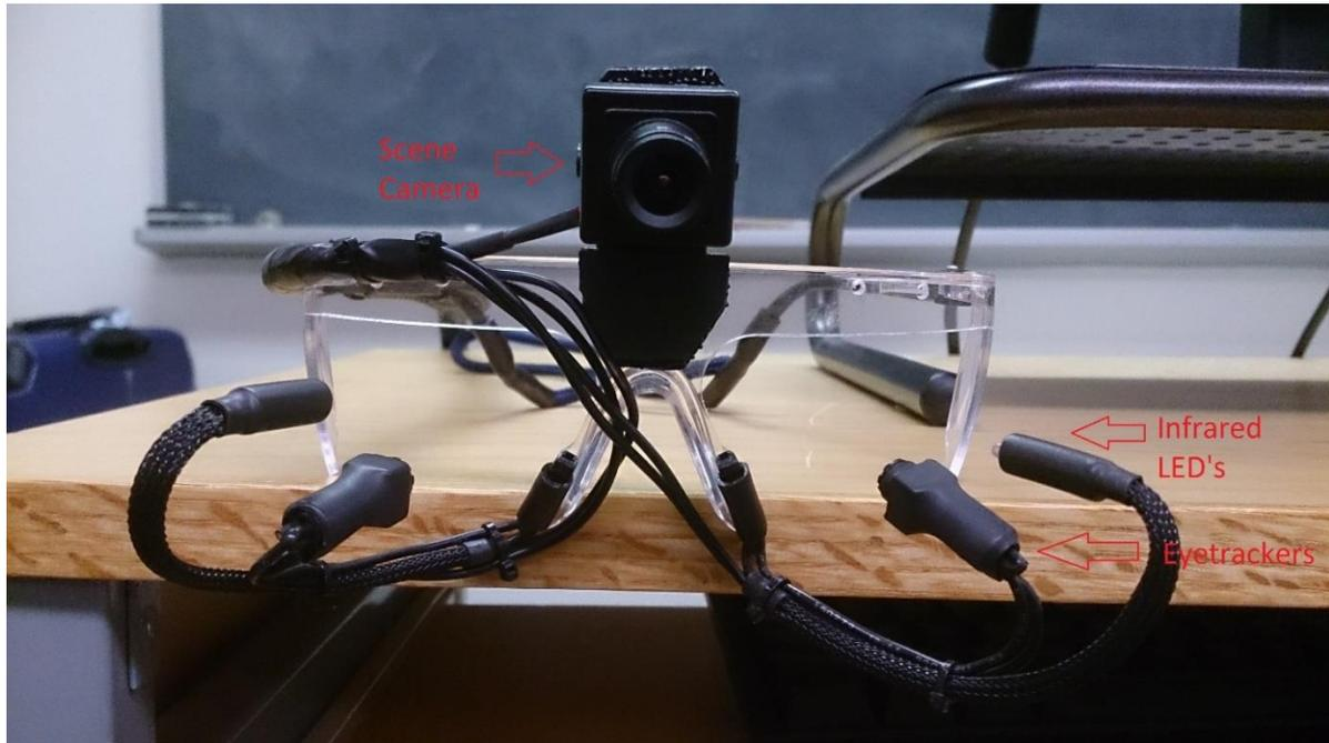
**Figure 2.2 Arrington eye tracker. Scene camera located above the nasal bridge; eye tracking cameras and infrared LEDs located in front of each eye**
