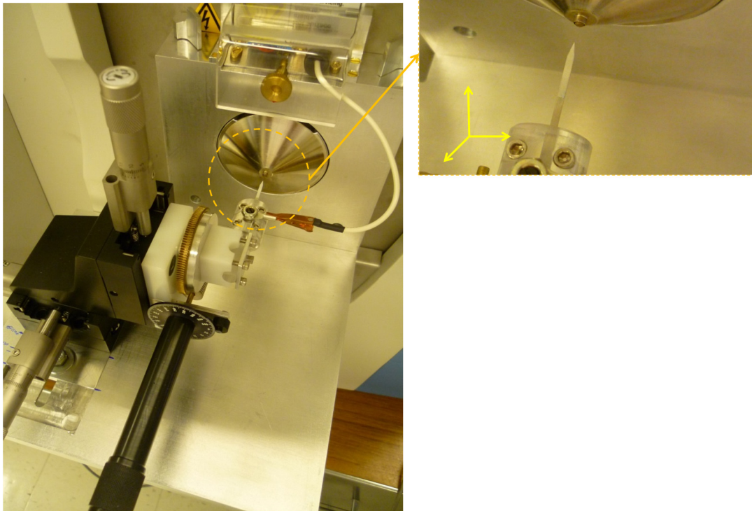
Figure 4.1 In-house ionization source for blade spray technology. The 3D-moving stage (Newport Corporation, Irvine, CA) not only adjust the position with a precision of 0.02 mm in each dimension (25 mm moving path), but also tunes the spraying tip at different angles on the Z dimension ( \pm 0.01^\circ per moving mark). In order to ensure optimum ion transmission, the position of the blade-tip should not be offset more than 2 mm in all directions from the centre of the ion-transfer capillary.
