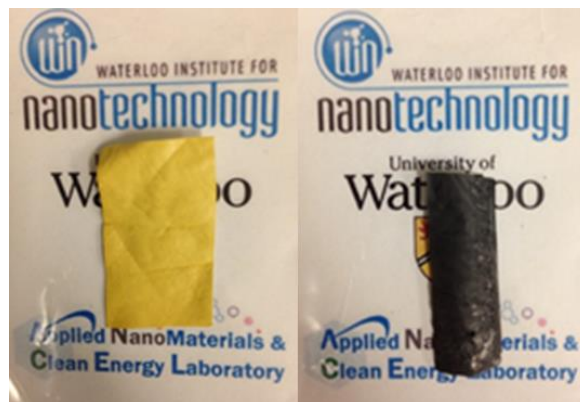
Figure 4- 4 Digital photos of porous PBI-Py film before (left) and after pyrolysis (right)
