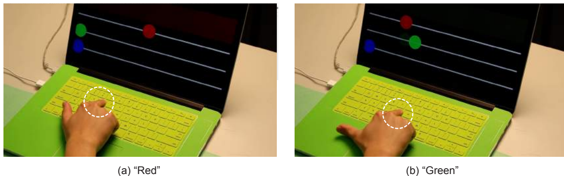
Figure 3.10: Simultaneous parameter control – pressing \text{R} , \text{G} , \text{B} with the right index finger and the thumb extended could achieve simultaneous parameter control of RGB colour values.
