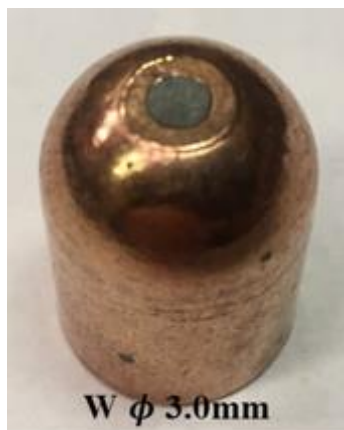
Figure 5.1 Schematic of modified inserted electrode
