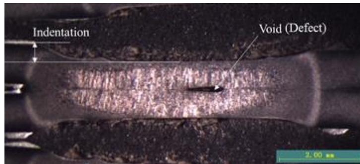
Figure 2.3 Weld defects of RSW weld
