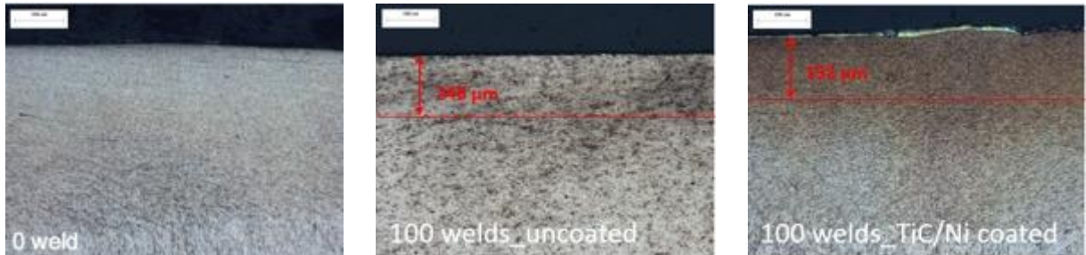
(a) Recrystallized depth of Class 2 electrodes
