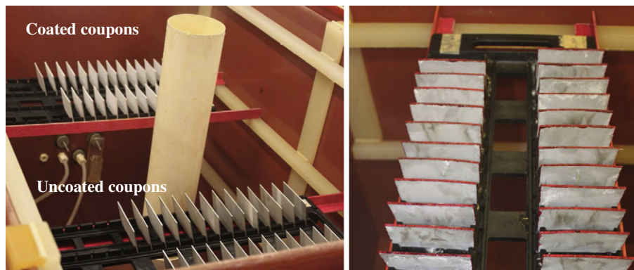
Fig. 5. The corrosion chamber (a) showing bulk and coated coupon distribution on racks before test, (b) edges of coated samples masked off by Microstrop lacquer mask.
