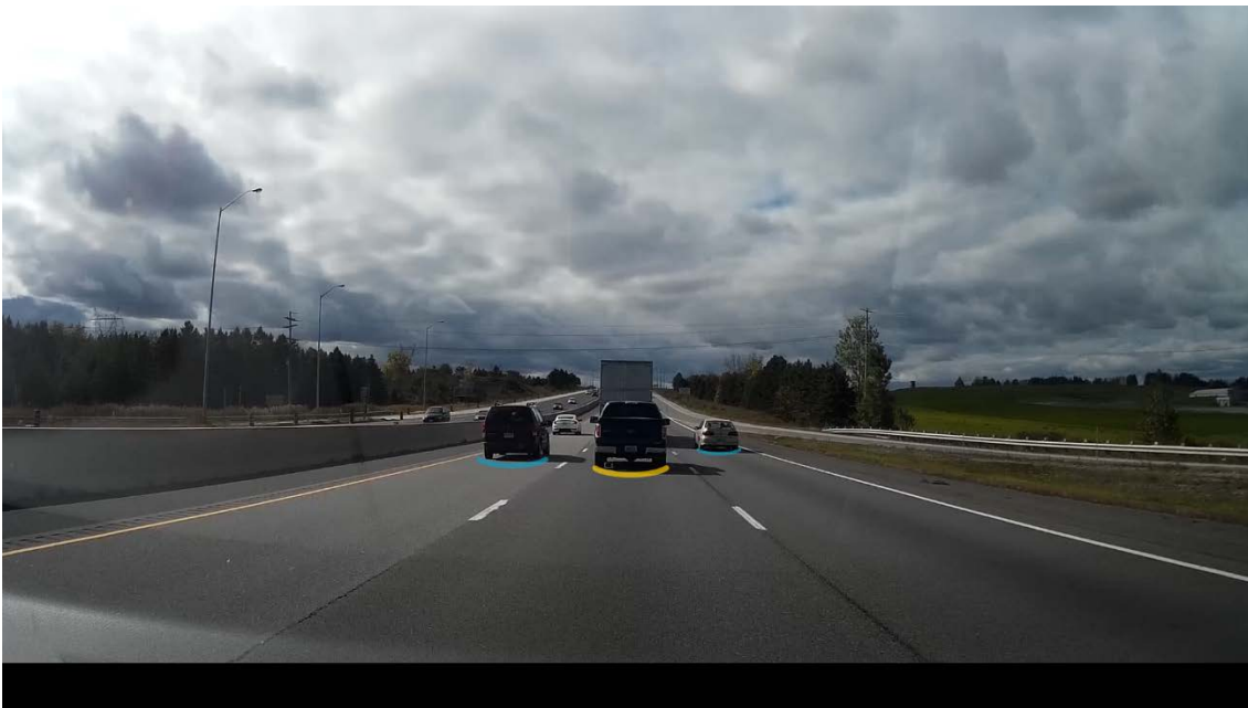
Figure 9. Advanced Display. This variation highlights lead vehicles and vehicles in other lanes.
