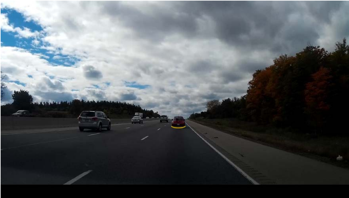
Figure 8. Basic Display. In this variation, only the lead vehicles (vehicles on the same lane as the own car) are highlighted.
