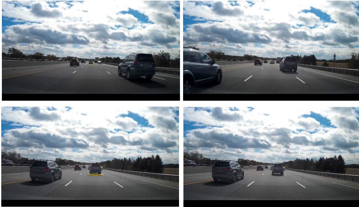
Figure 11. AR HUD failures. This is one of the examples where the reliability of AR HUD was manipulated. On top two images, the vehicle on the right moves into the middle lane. On the bottom left, the vehicle identifies it as a lead vehicle and highlights it. On the bottom right, the vehicle “fails” to identify the lead vehicle. Hence, no highlighting occurs.
