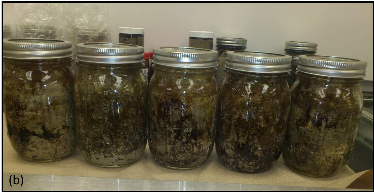
Figure A-2. Impacted aquifer material samples used for (a) slurry experiments and the “bleb” architecture physical model experiments, and (b) the “saturated lense” architecture physical model experiments.
