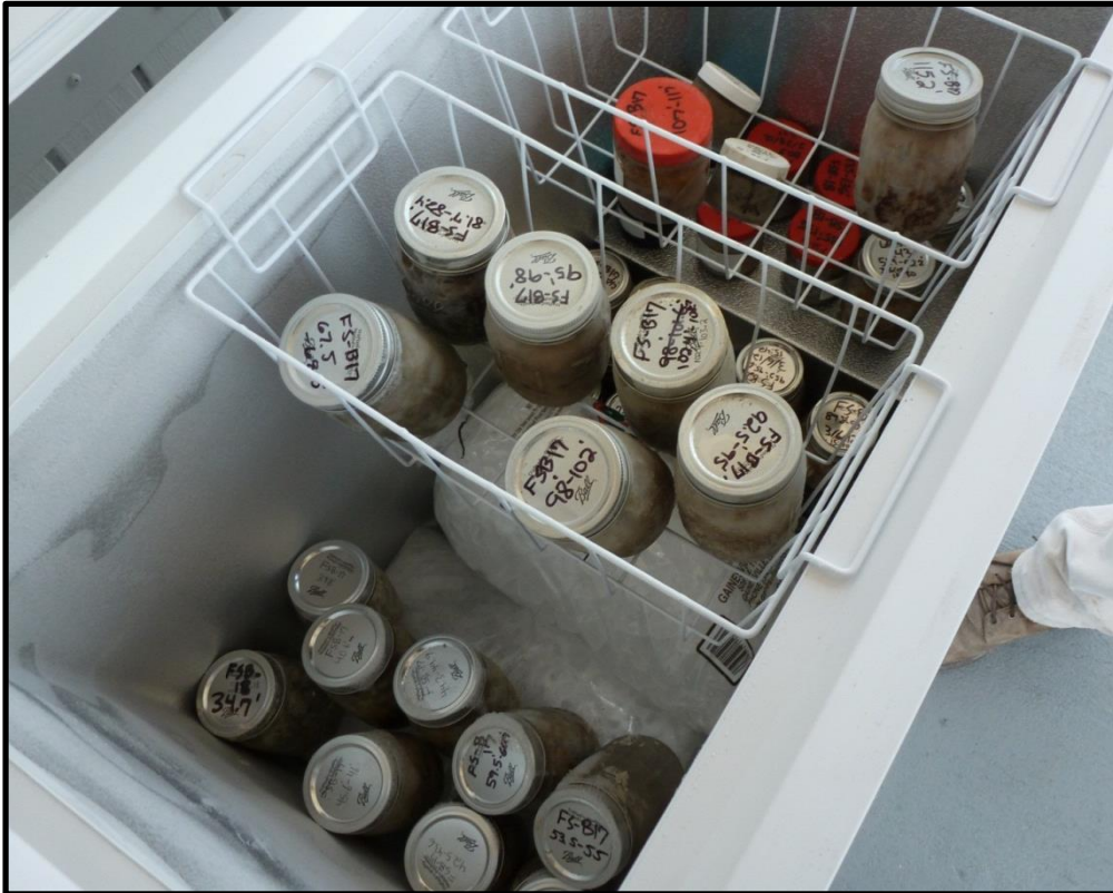
Figure A-1(a). Image of impacted core materials from the weathered limestone unit stored on site in freezer.
