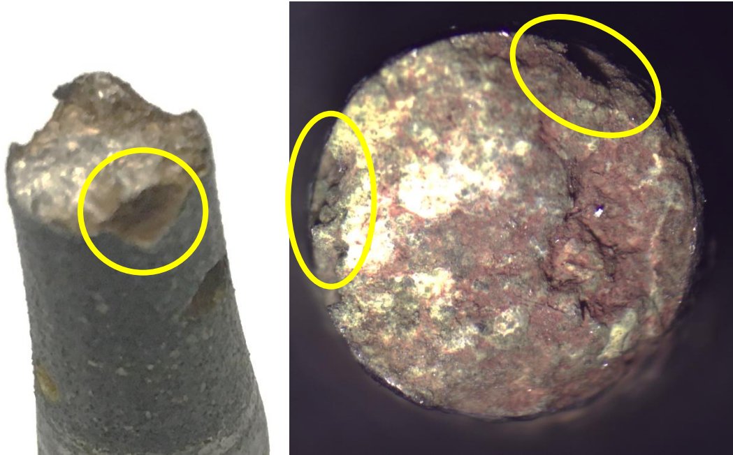
Figure 5-12: Fracture surface happens in pitting holes location
