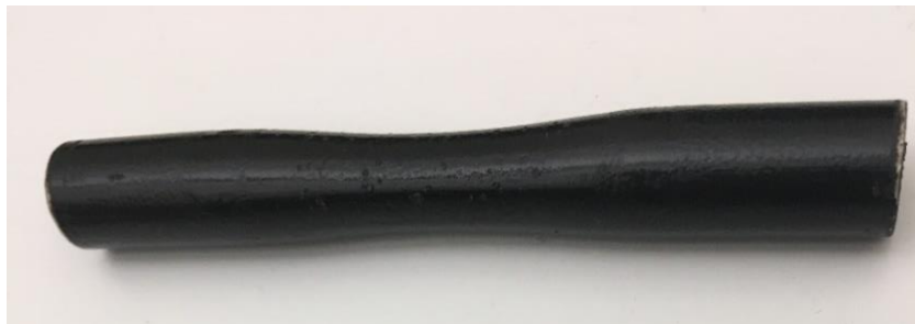
Figure 5-17: A cold spray coated e-painted sample after 10 million cycles in 80 MPa
