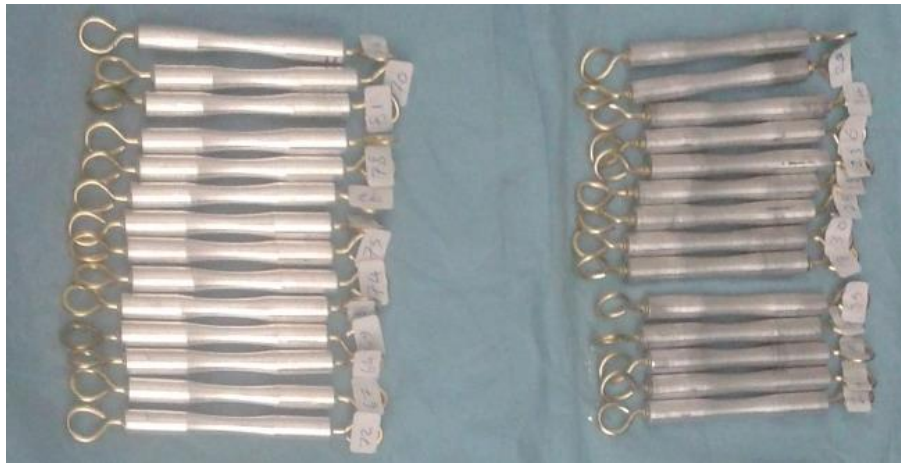
Figure 5-4: Samples prepared for electrostatic painting. Bare samples (left) and cold spray coated polished samples (right)
