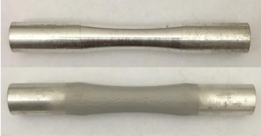
Figure 4–4: Un-coated sample of AZ31B (top) and coated sample by cold spray of Al 7075 (below)
