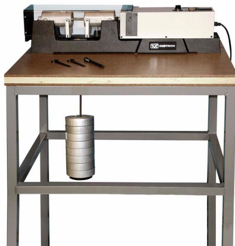
Figure 4-7: Rotating-bending fatigue test device [63]
