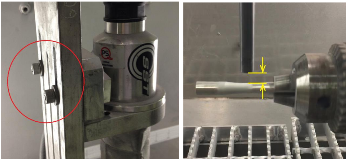
Figure 3-6: The adjustment of the nozzle vertical position (left) and the stand-off distance (right)
