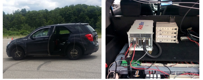
Fig. 10: 4WD SUV test platform and I/O layout
