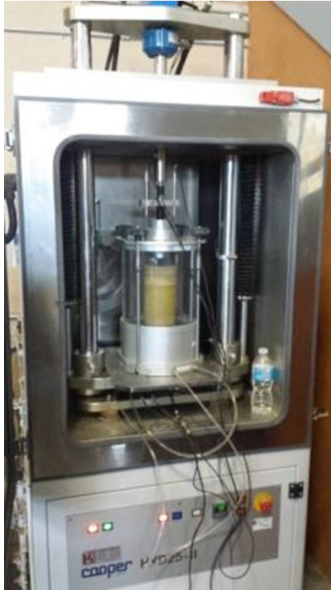
Figure 5-4. Triaxial resilient modulus testing apparatus at Lafarge Canada ITC
