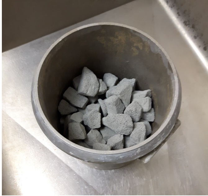
Figure 10-10. View of a dry sample of material LWA-B in the density testing apparatus
