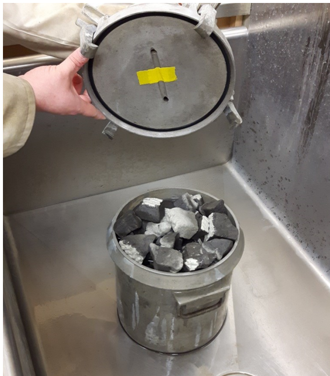
Figure 10-11. View of a sample of material LWA-A after immersion during density testing
