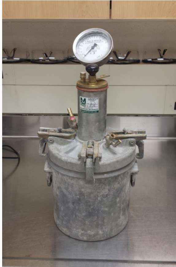
Figure 10-9. Concrete air void testing apparatus used for relative density measurements
