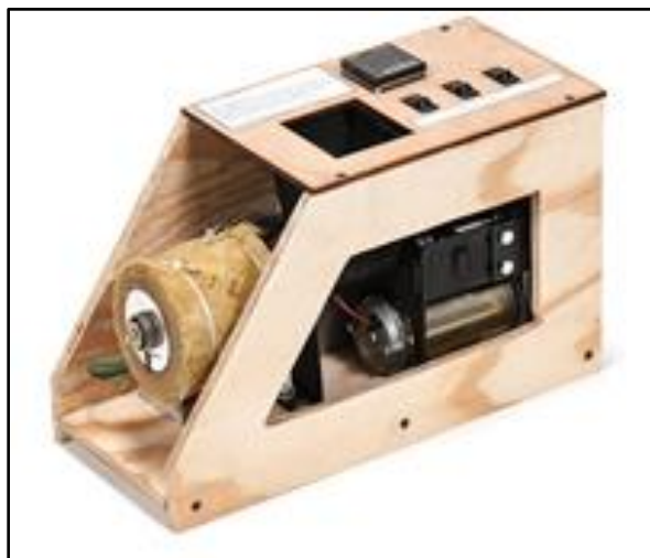
Figure 3-2: Filabot wee single-screw extruder
