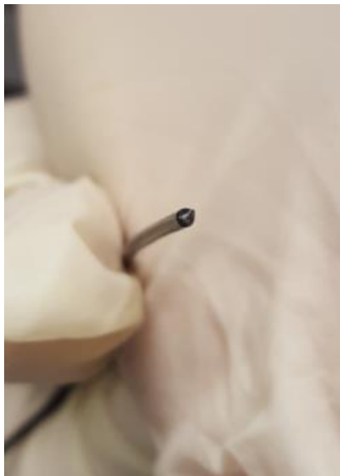
Figure 4-22: Cross-sectional view of the filament shows good ovality
