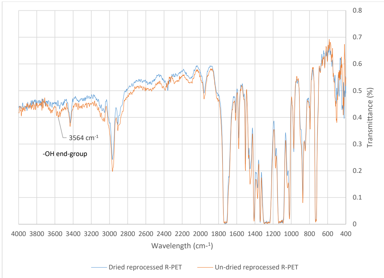
Figure 4-14: FT-IR spectrum of reprocessed R-PET dried and undried prior to extrusion
