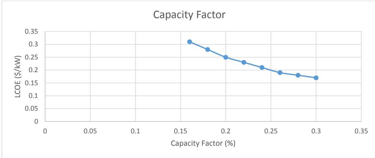
Figure 27. LCOE for Solar PV with different capacity factor values
