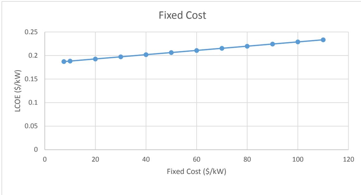
Figure 28. LCOE for Solar PV with different values of fixed cost
