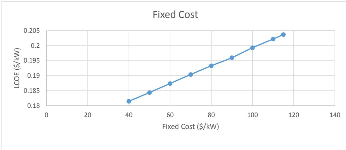
Figure 24. LCOE for Solar CSP with different values of fixed cost
