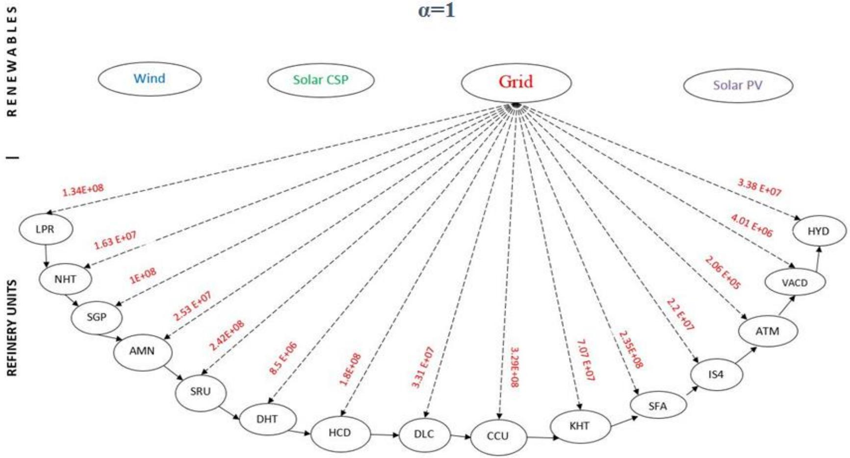
Figure 15. Superstructure for Energy Resources Distribution and Refinery Units at an  $\alpha$  value of One
