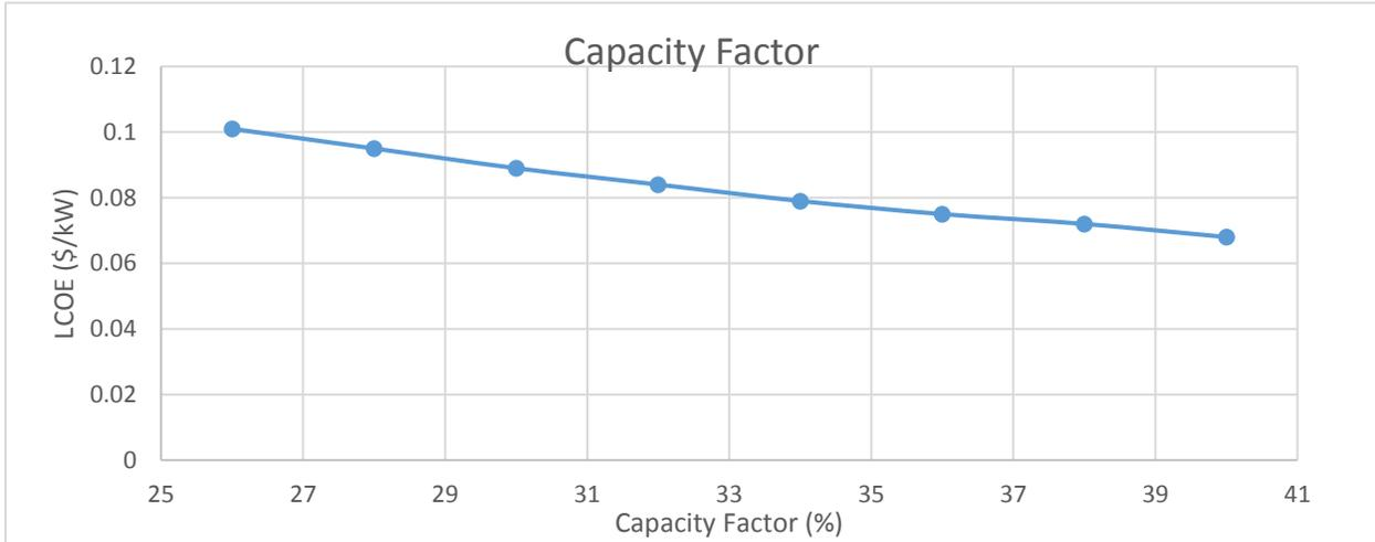
Figure 30. LCOE for Wind energy with different values of capacity factor
