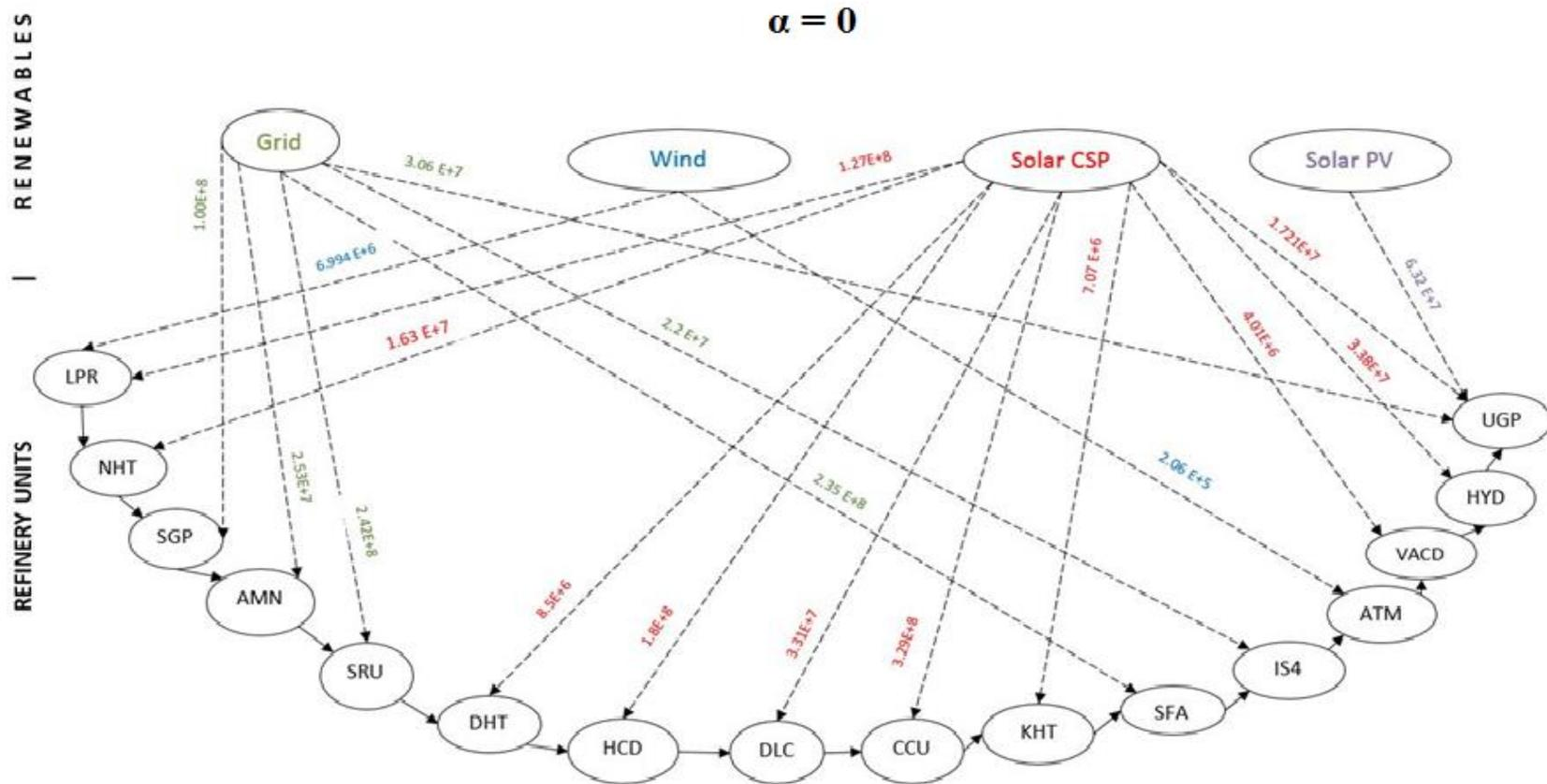
Figure 13. Superstructure for Energy Resources Distribution and Refinery Units at an  $\alpha$  value of zero.
