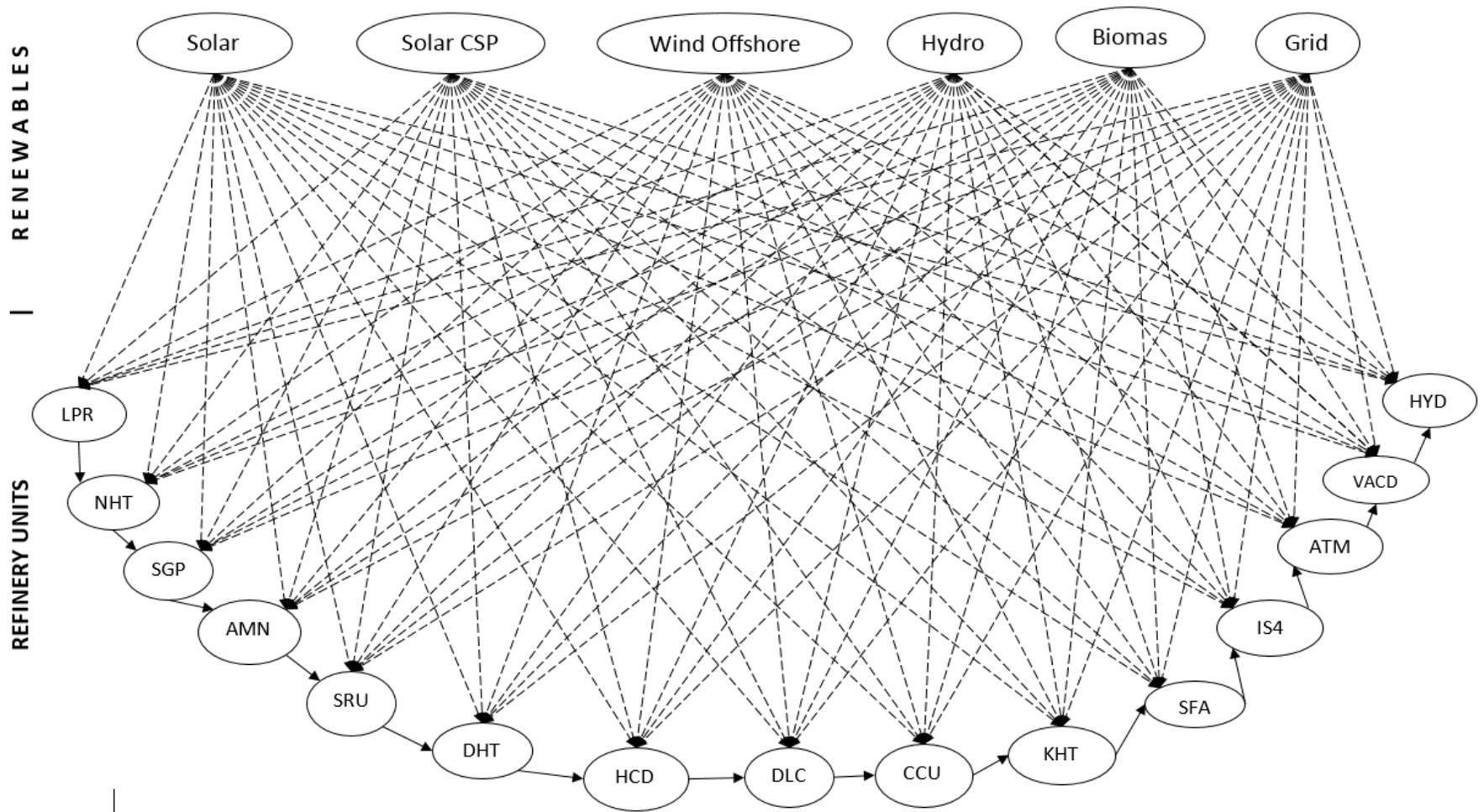
Figure 6. Superstructure diagram for the crude oil refinery units connected with all available energy resources.
