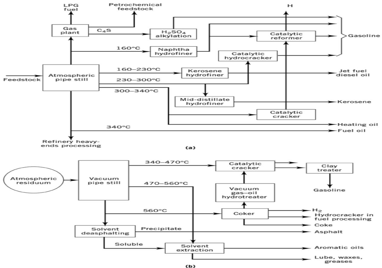
Figure 4. Typical Crude Oil Distillation Unit Flow Diagram [10]
