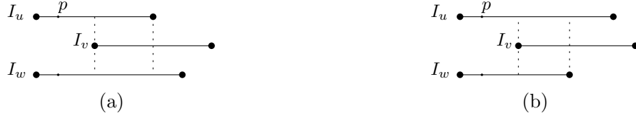
Figure 3.2: If u protrudes from v on the left, Figure 3.2a shows that if r(I_u) < r(I_w) , then s(u, w) is as large as s(u, v) plus one additional point p outside I_v ; Figure 3.2b shows that if r(I_u) \geq r(I_w) then s(u, w) is as large as s(w, v) plus one additional point p outside I_v ; in both cases w satisfies the condition for (u, v) \in R_s
