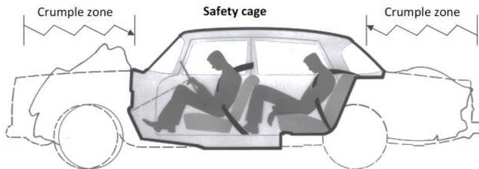
Figure 8: The major crash management zones of a vehicle [21]
