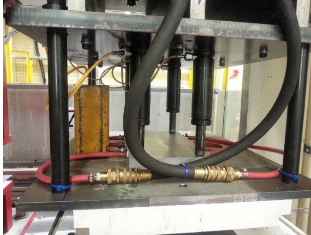
Figure 24: Cooling block and nitrogen springs installed in upper die
