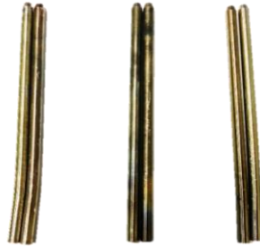
Figure 23: Warped ejector pins
