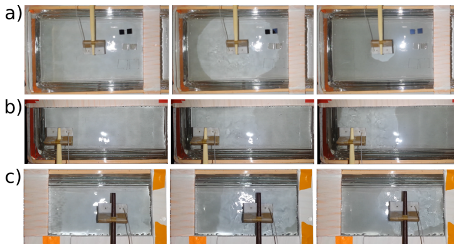
Figure 5.2 Macroscopic view of film formation of TEGO film by barrier-free at various condition: Snapshots of videos recorded through TEGO deposition by setting the dripping position at the center (a) and close to one side of the trough (b, c) from two typical concentrations: 0.025 mg/mL (a, b) and 0.1 mg/mL (c).
