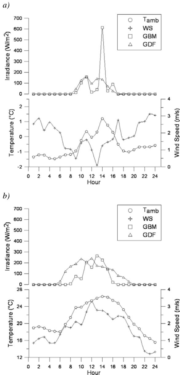
Figure 4. Hourly beam (GBM) and diffuse (GDF) irradiance (Kotey and Wright (2006)), ambient temperature ( $T_{amb}$ ) and wind speed (WS) on a south facing window- a) winter day - Jan 01, 2004, b) summer day – July 01, 2004.
