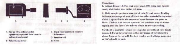
Figure 4 Keyes openness measurement apparatus (Keyes 1967).
