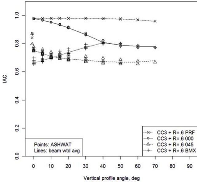
**Figure 5** IAC versus solar profile angle, indoor medium colored venetian blind, four types of slat-angle control. Note: Slat angle – PRF: follows profile angle (maximum gain); 000: horizontal; 045: 45 down; BMX: slat angle adjusted hourly to exclude beam (maximum slat angle = 0°, hence convergence with 000 curve).
