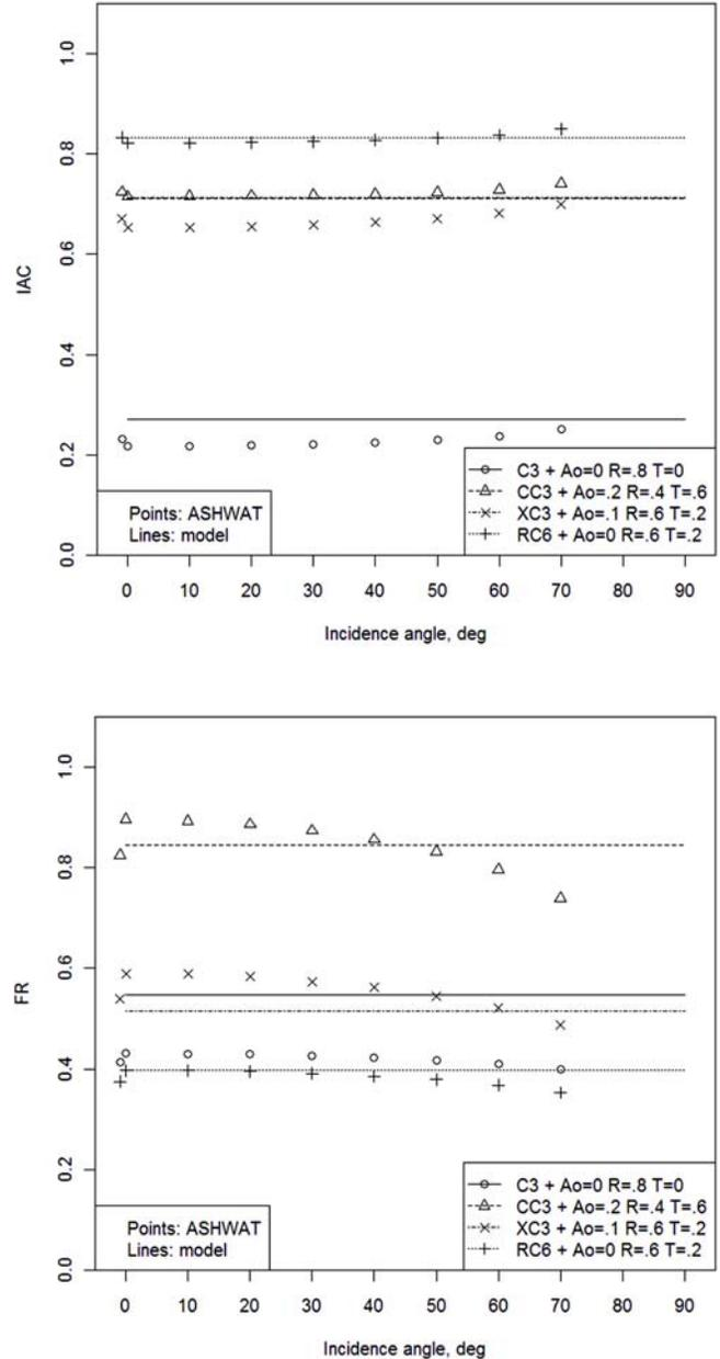
**Figure 4** Roller blind example model fits: IAC (upper) and FR (lower). Notes: Glazing -- C3: single clear 3 mm; CC3: double clear 3 mm; XC3: double selective low-e 3 mm; RC6: double reflective 6 mm. Ao = openness; R and T as defined in Table 1.
